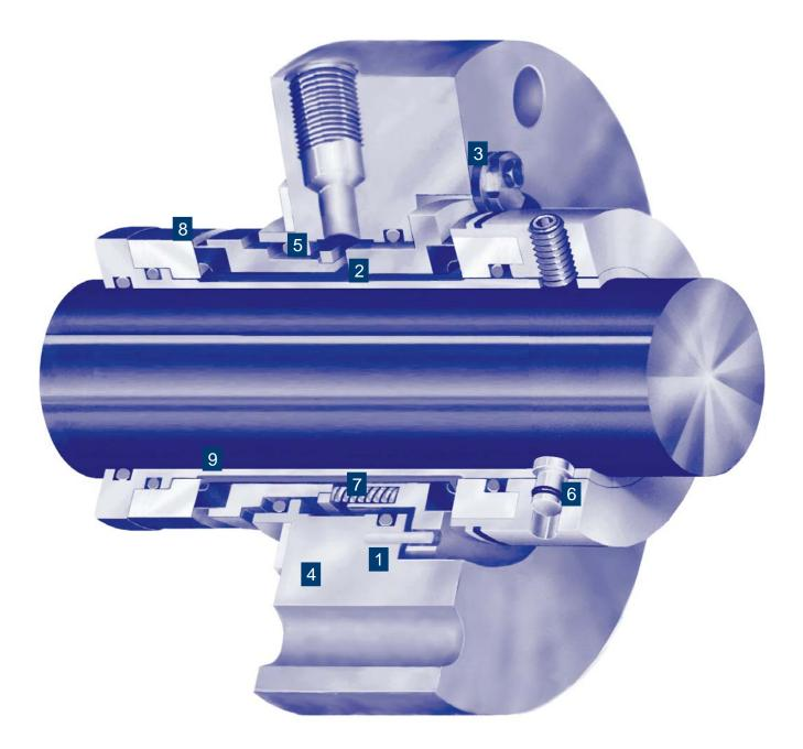
The ASI Model 600 is specially engineered to withstand greater radial and axial movement common to larger equipment such as slurry pumps, mixers and agitators. The seal components are designed to work in unison, preventing under or over-compression of the seal faces, as well as increasing free movement of the seal.
